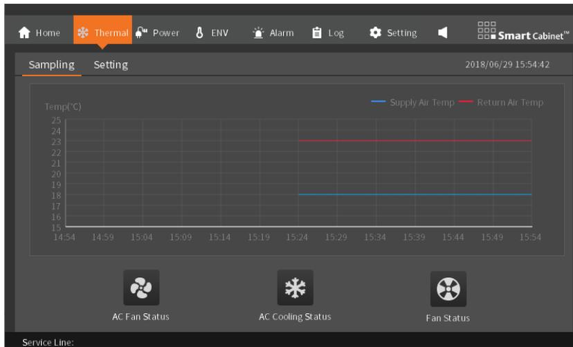
Figure 3-3 Thermal management data collection screen
